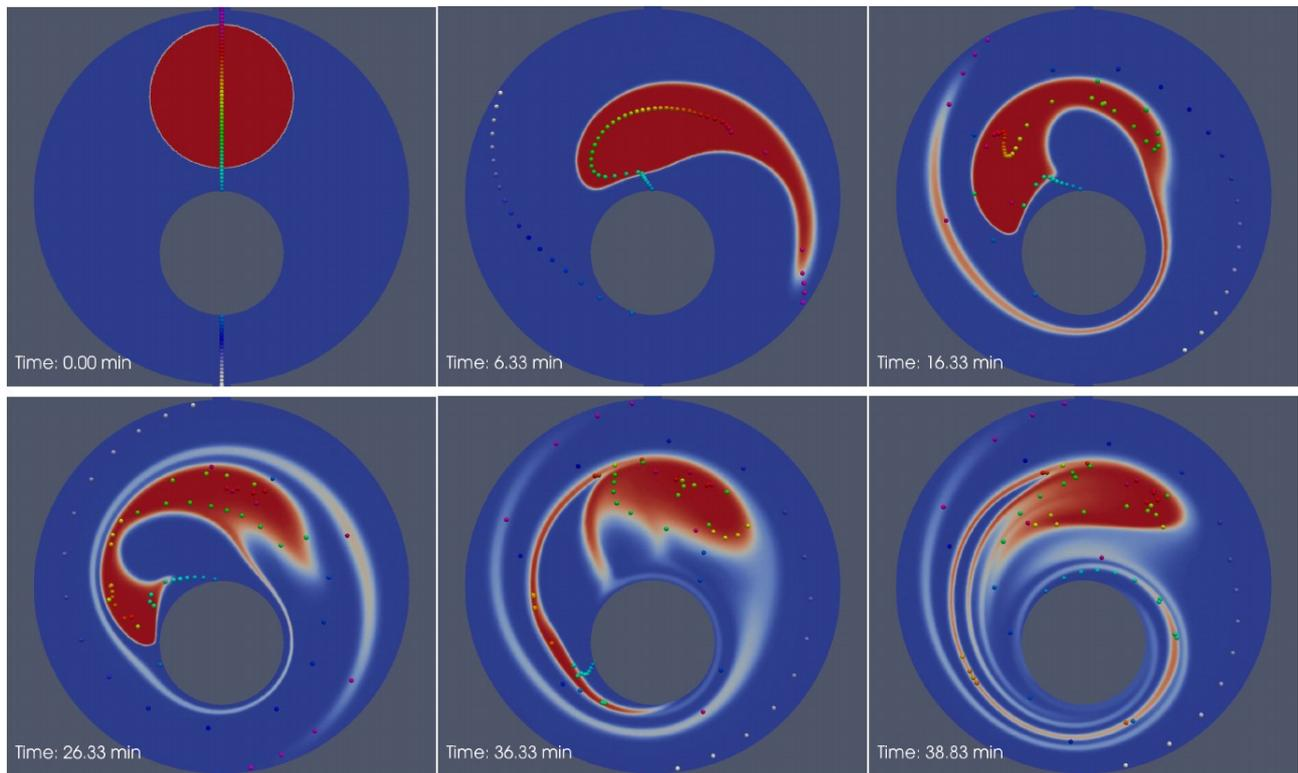
Fig.1 – Snapshots at different times for the simulation of the magma mixing experiment [Morgavi et al., 2013] considered for the validation of MF. As observed in the experiments, the basaltic (low viscosity, red) and rhyolitic melts (high viscosity, blue) mix through a stretch and fold mechanism due to the independent rotations of the outer and inner cylinder walls of the mixing device. Fluid tracers (colored particles) are also added here to better visualize the evolution of the mixing process.
