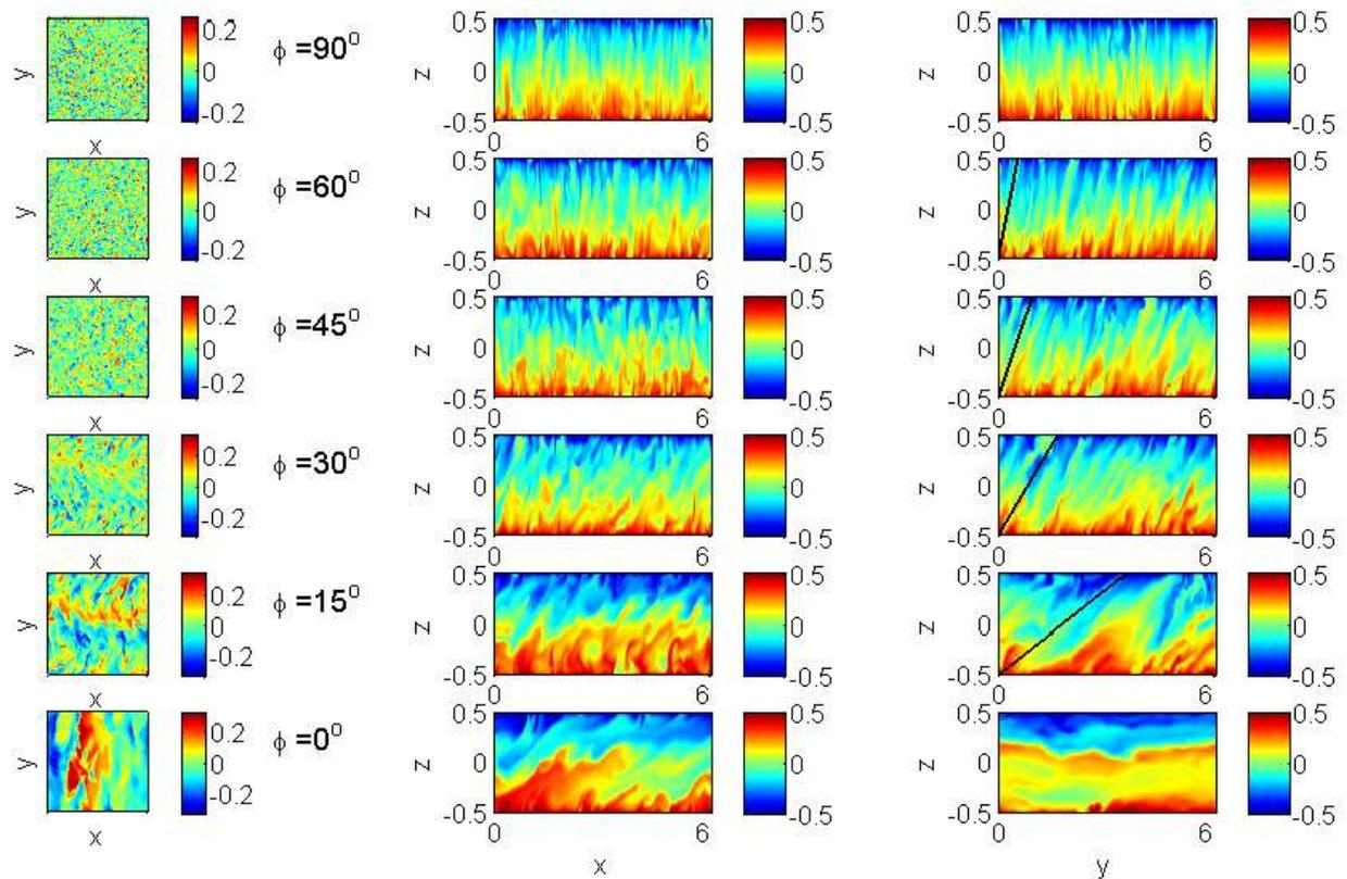
Fig.1 – Horizontal (left column) and vertical (central and right columns) sections of the temperature field computed at statistically stable state, at mid depth and mid width. The rotation axis resides on the y-z plane and its orientation is represented by the black line in the third column panels. The convective plumes align with the rotation axis on the y-z plane at each latitudes.
