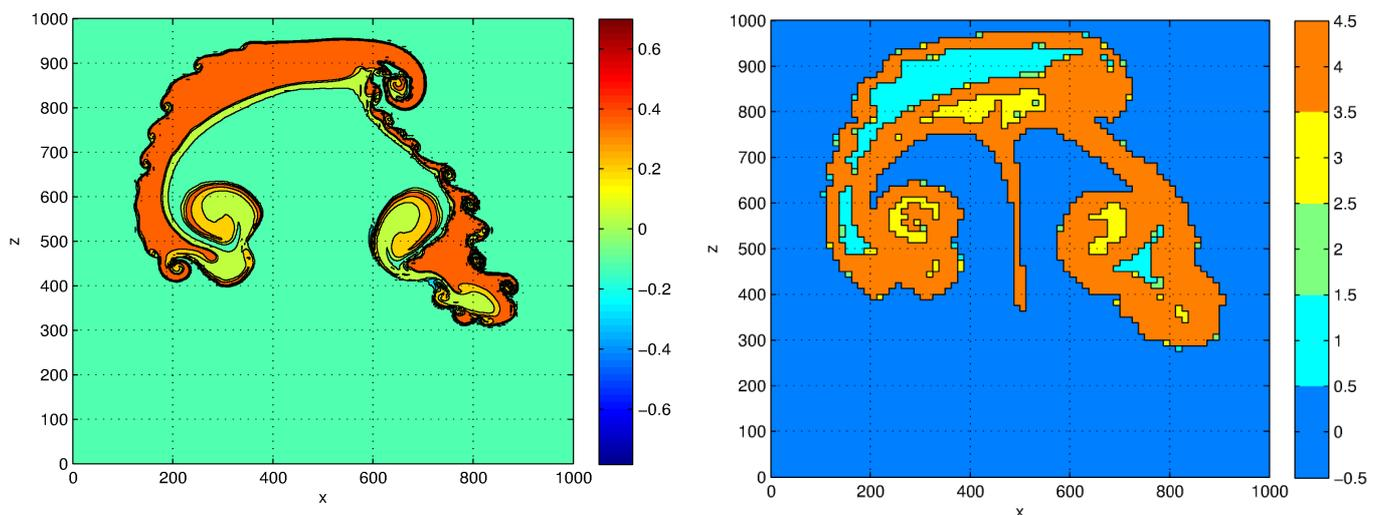
Fig.1 – Double bubble test case (Robert 1993): potential temperature (left) and local polynomial degrees for potential temperature (right).
