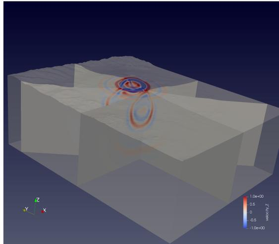
Fig.1 – Numerical seismic ground motion propagation (velocity) on the vertical component for a dipole source placed under Mount Etna (Sicily). The unstructured grid, built with the internal mesher of SPECSEM3D, is made of 173 568 spectral elements and includes topography and the 1D velocity model of Chiarabba et al. (2000). Simulation has been run on the A1 partition of Marconi CINECA HPC resources on 96 cores.
